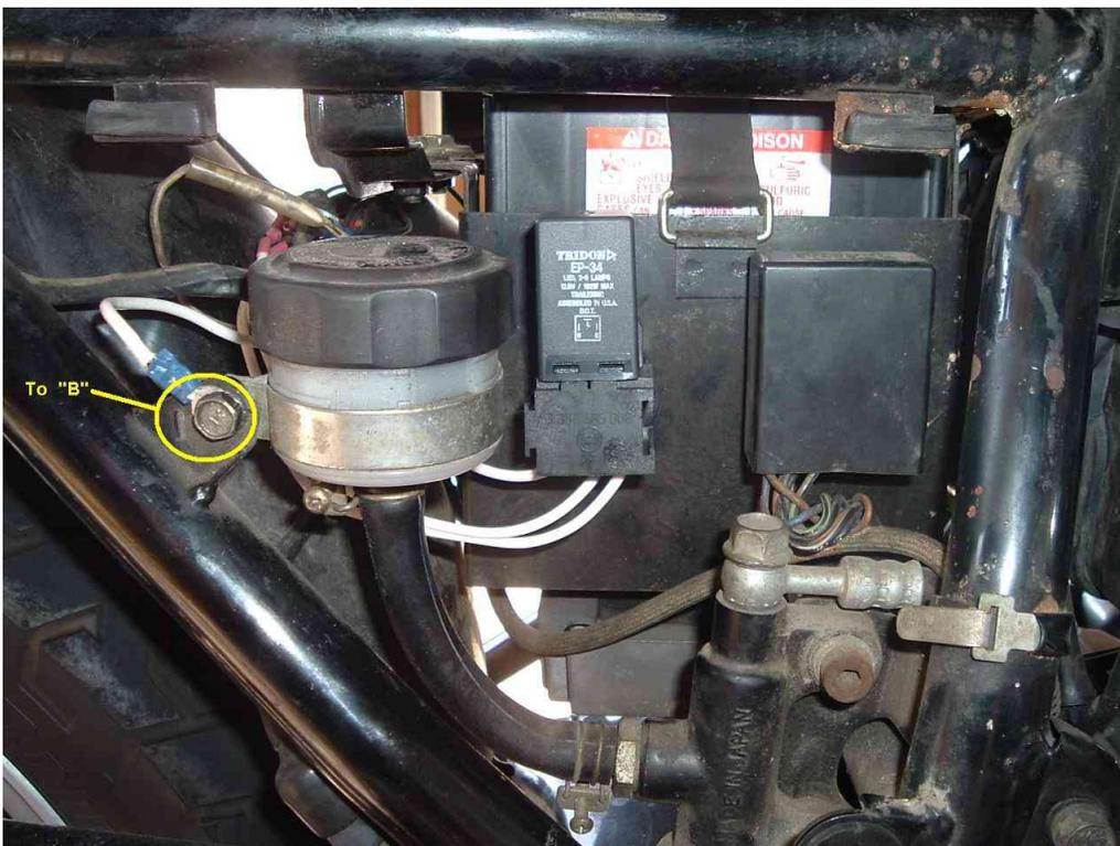
I also put a zip tie around the relay and the mounting tab to help hold it in place and guard against vibration.
