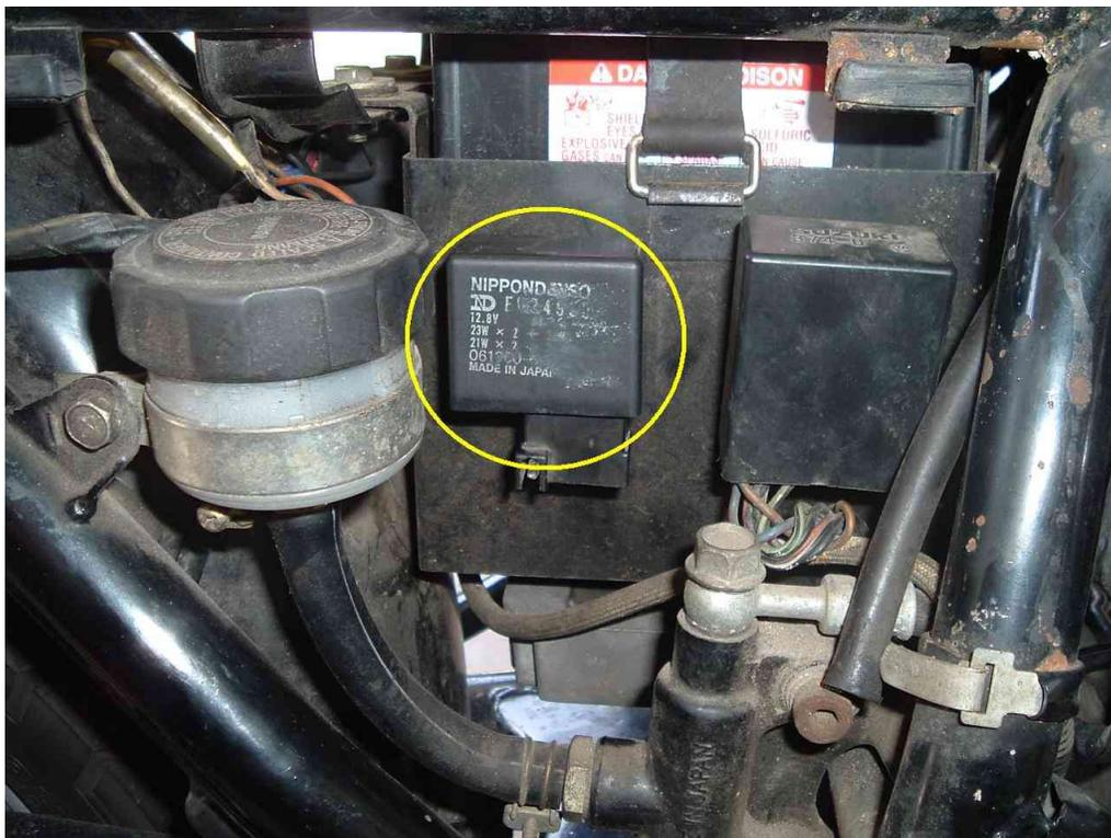
Following Mr. longgreensilverado's advice, I purchased a Tridon Stant EP34 electronic flasher (\$10 or less). A relay socket is optional, but it came in handy for mounting the relay. The socket I purchased is a Bosch style 4 or 5 terminal socket made by Motormite, part# 85170. If you don't use the relay socket, you will need some female blade connectors to wire up to the blades of your flasher unit.
