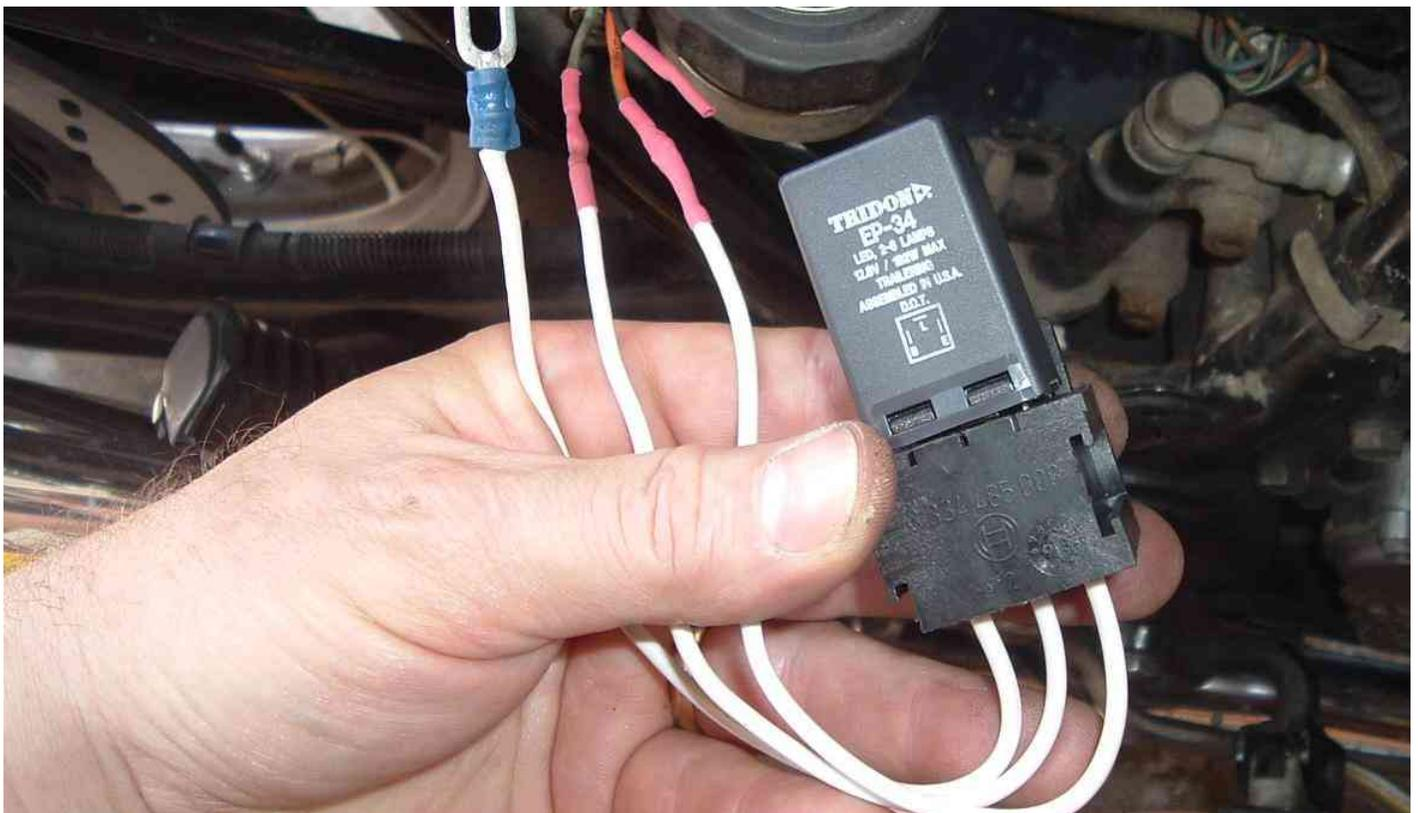
Now. Where to put this thing? It wouldn't just clip on the battery box like the old unit. So I made a slight modification. Since the socket had a mounting hole, I decided to drill the tab for the old relay to make room to bolt it on the existing tab.
