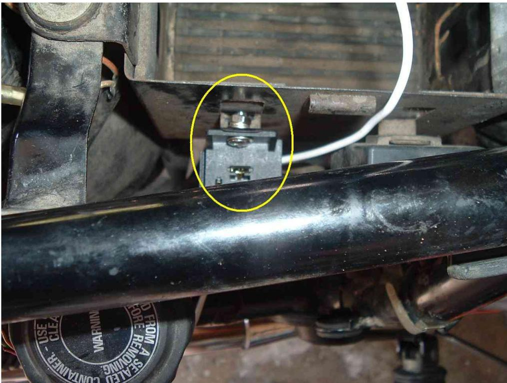
Here is a view of the socket from the right side. One wire is pointing up because I was thinking about connecting the relay's ground wire to the (-) battery, but it wasn't long enough.
