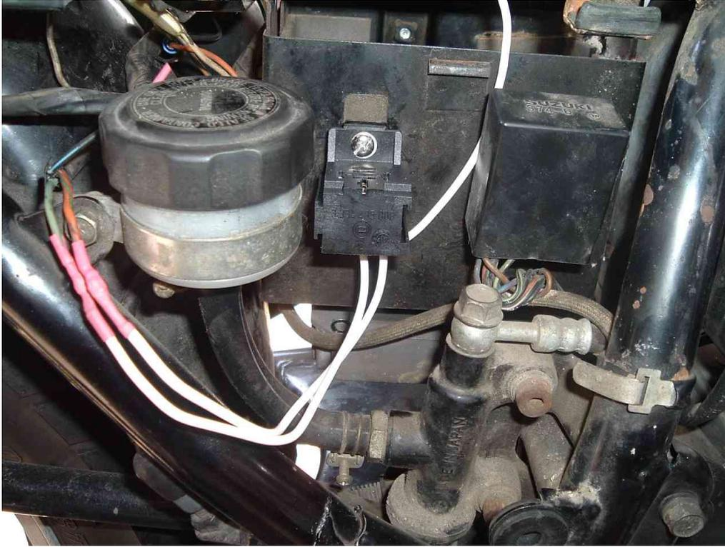
Instead, I connected the relay's ground wire to the frame mounting bolt for the rear brake master cylinder.
