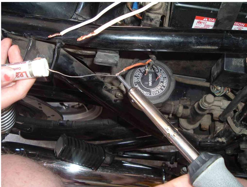
After tinning, I have crimped a spade connector on the ground wire and put shrink tubing in place to cover the soldered connections. I put shrink tubing on the Blue/Black wire just to cover and protect the end.
