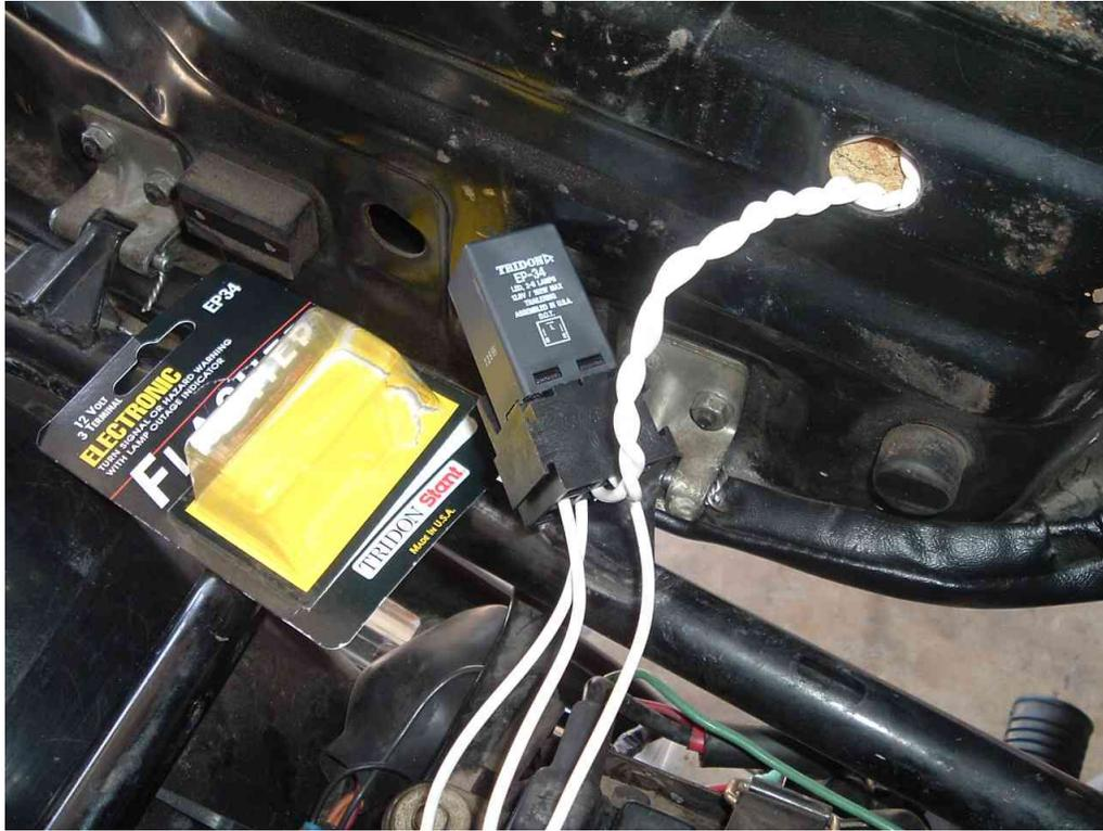
Below, I am testing my connections to make sure the relay will flash the turn signals.
