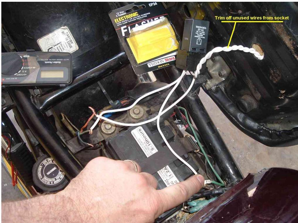
The (switched) 12v Orange/Green wire gets connected to the 'E' terminal on the relay. The light blue (actually it looked more like a faded green color) drive wire to the lamps gets connected to the 'L' terminal of the relay. The 'B' terminal of the relay gets connected to frame ground. Please note that I am leaving the Blue/Black wire disconnected. This will disable the auto-cancelling feature of the turn signals.
