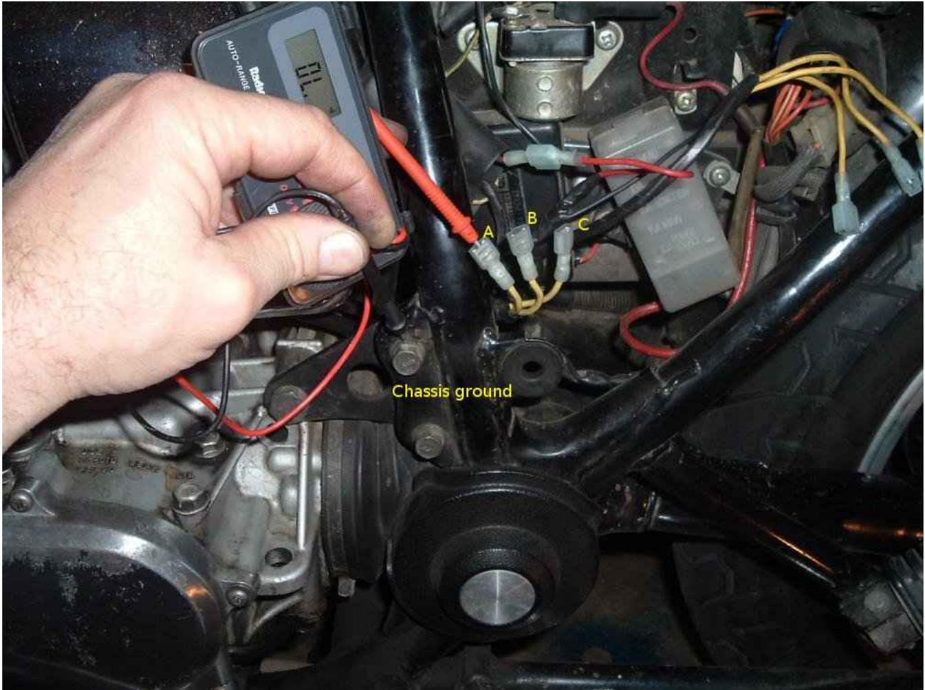
My meter reads "OL", meaning "over limit", when there is no connection or infinite resistance between two points. Let's hope yours reads the same when you perform this test. But it has also been my experience that even after passing these first two tests, the stator may still be bad.
