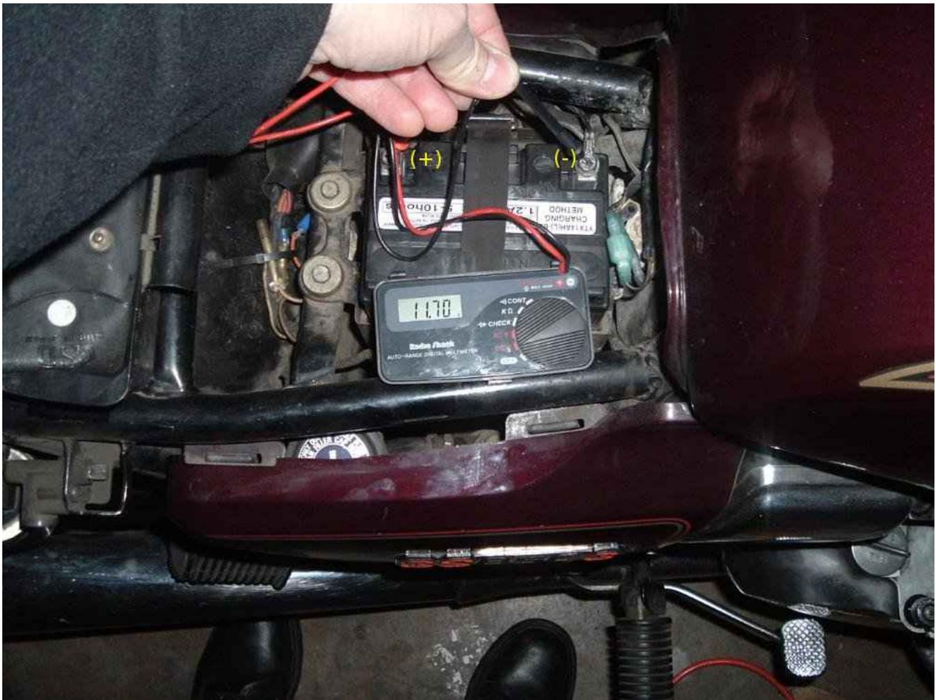
With the motor at idle you should see around 13 volts or better. At 4000 rpm you should see around 14.5v. As you can see, this motorcycle has a problem with its charging system.
