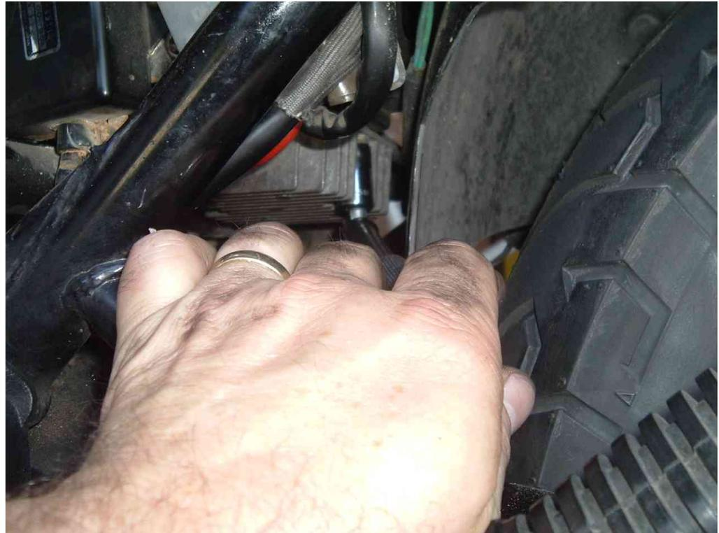
Usually what I end up doing is using the socket driver just to loosen the bolt a little. Then I will take the socket and a short extension to finish the job as illustrated here on the bolt nearer the engine (*really hard to get to*).
