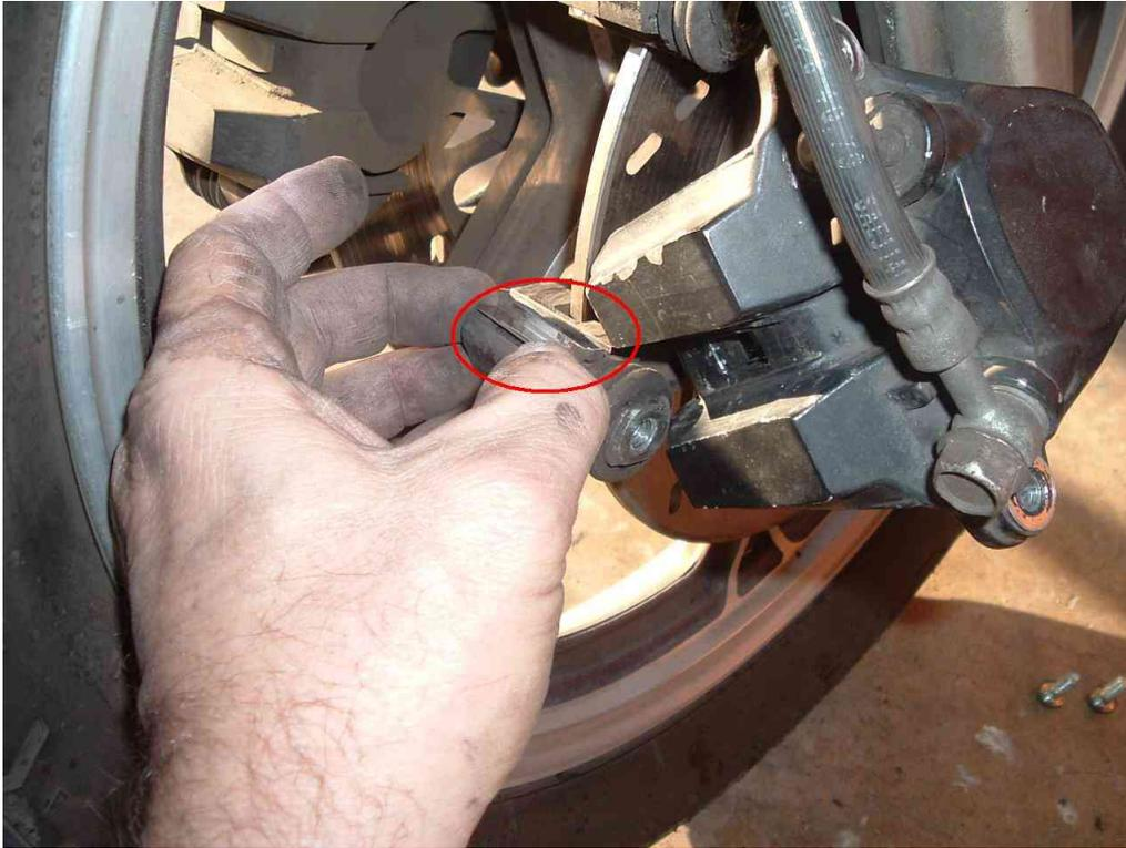
Next, let's clip the shim pad back on the new brake pad. This brake pad goes on the outside of the assembly, next to the brake piston.
