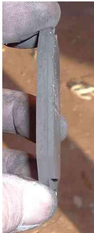
Let's begin our reassembly. First, I put a guide pad on the bottom, the wide edge laying on the bottom of the caliper bracket.
