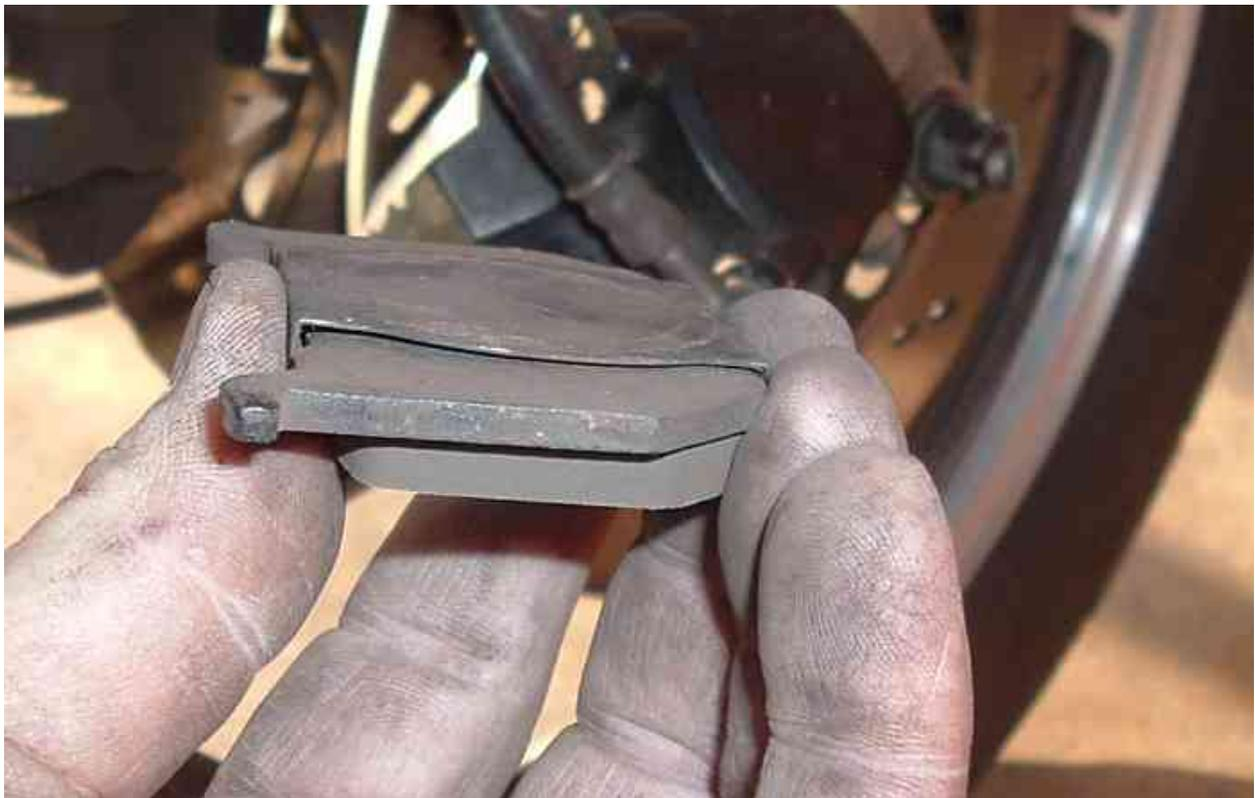
Now it starts getting a little tricky, only because you have to hold several parts in place at once. Start by squeezing the brake piston back into the cylinder to give us room for the new pads. Put the upper guide pad in place (in red), wide edge against the top of the caliper bracket.
