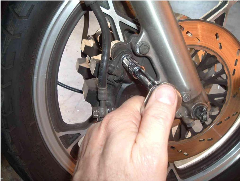
Once you have these two bolts removed, take care as you slide off the caliper. The brake pads and various clippy things will fall out. Here is a picture of how the parts are arranged under the caliper.
