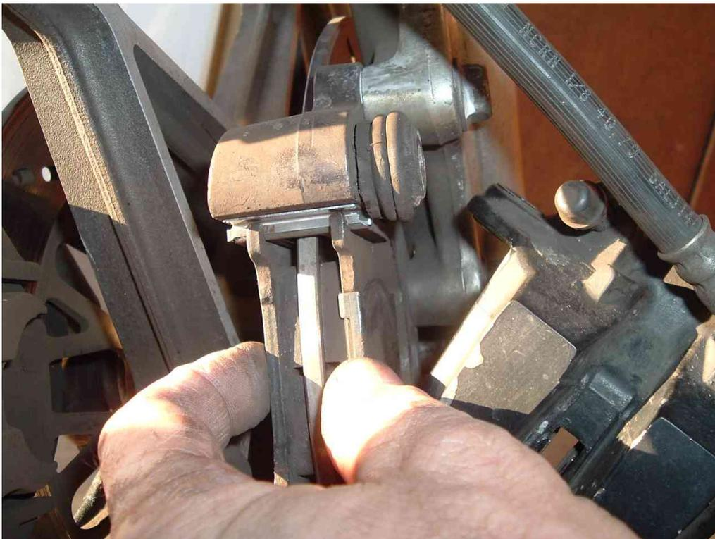
Now slide the caliper assembly in place, being careful not to dislodge the spring pad. Use a couple of fingers to hold the inside brake pad while you push the caliper with your thumb. If you are not taking a picture, you could actually use both hands for this.
