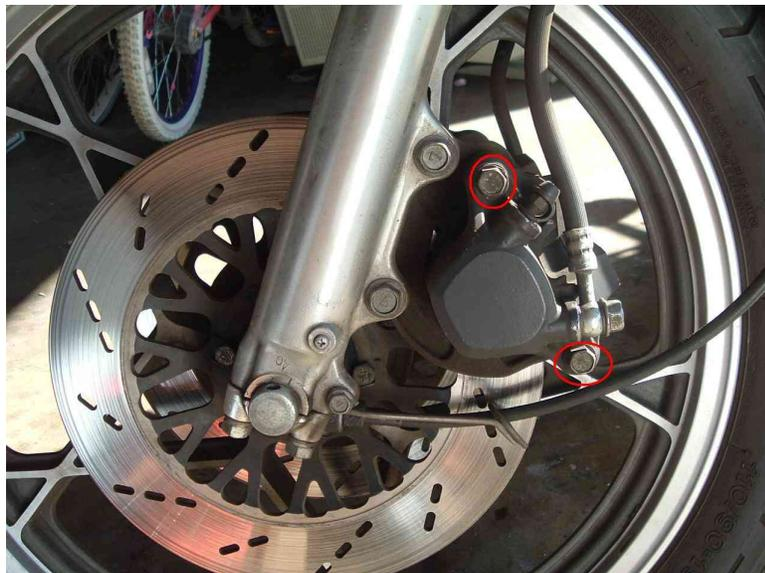
Remove the two 12mm bolts holding the caliper assembly.
