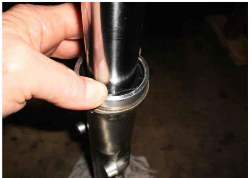
Now we can put the dust seal back on and replace the fork oil. Most of the time you'll use a 10wt oil but 15wt can be used for heavier loads or for a stiffer ride.
