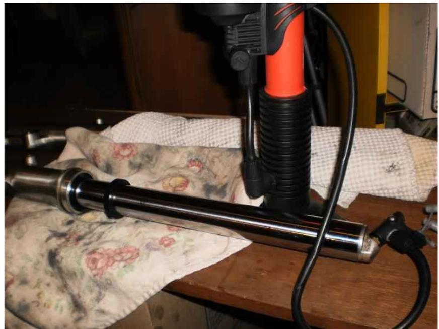
Now we can put the new seal in place and slide it down the fork tube. Make sure to orient the seal properly. The open edge with the coil spring band should face the bottom of the fork.
