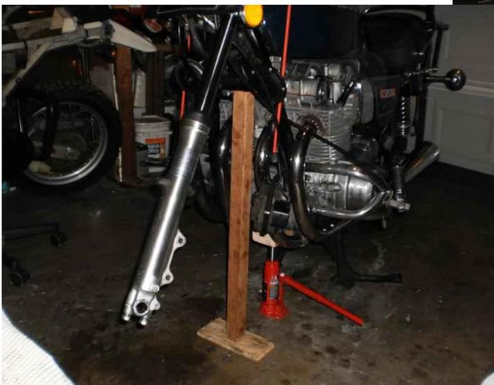
...as well as a 2x2 supporting the front of the frame under the steering head.
