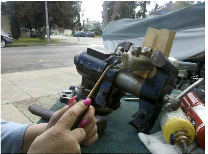
I bought some special snap ring pliers to remove the retainer clip, but these weren't really necessary. I also purchased a special fork seal puller but didn't get a chance to use it. Maybe next time.
