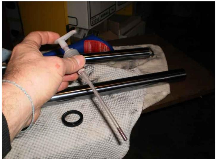
After dumping in the oil I pump out the excess. I place the bottom of the pump cap on the top of the fork tube. As I pump, the oil level goes down to exactly 140 mm. The important measurement is to make sure the fork oil level is within 1 mm between the two fork tubes. Using the pump on both forks ensures this.
