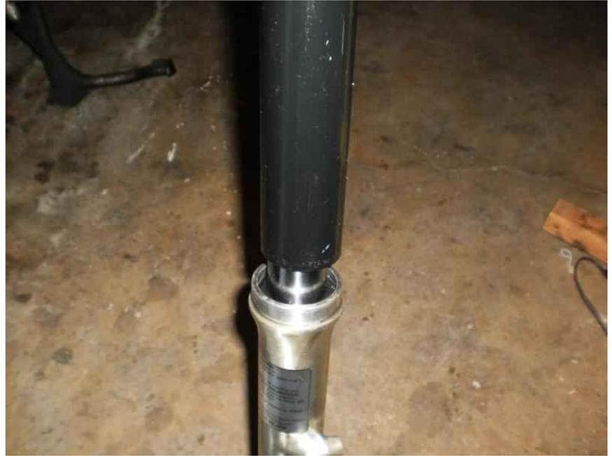
You may have to turn the fork upside down so that the PVC pipe is on the floor and you can push down on the bottom of the lower fork tube. This should seat the seal in place. This works better than trying to pound the seal in from the top.
