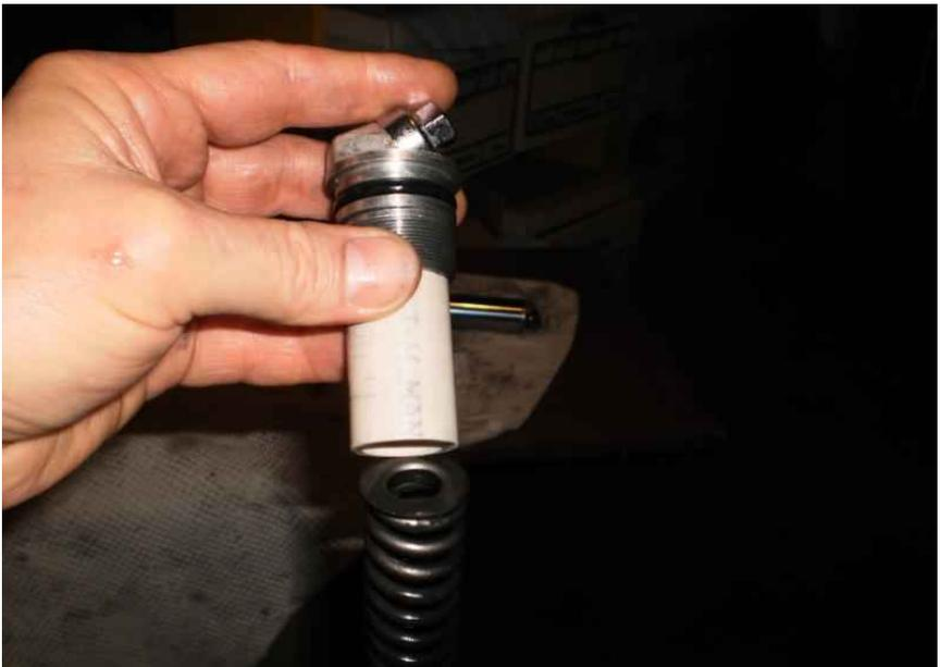
Lift the fork tube and screw the cap back in. This may take some special effort if you have long spacers. You may even have to put the tubes back in the triple tree clamps first.
