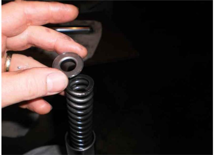
On top of the spring washer goes the spacer, and the fork cap, in that order.
