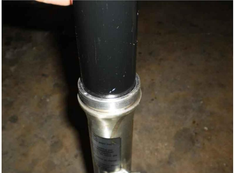
Once the seal is in place we can install the (new) retaining clips. Make sure they fit in the proper groove.
