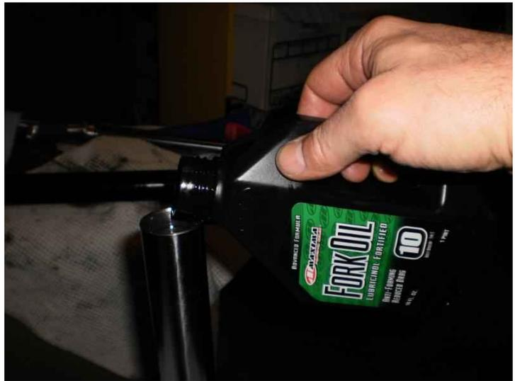
So I pour in about a cup of oil and use another special tool to measure 140 mm from the top of the compressed fork. As you can see, my special tool is a pump from a hand lotion bottle that has been cut to 140 mm in length (from the bottom of the cap).
