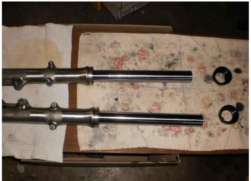
At this point, if we were completely disassembling the forks, the dampener rod bolts on the bottom of the forks would be removed. Unfortunately, my bolts were stuck hard.
