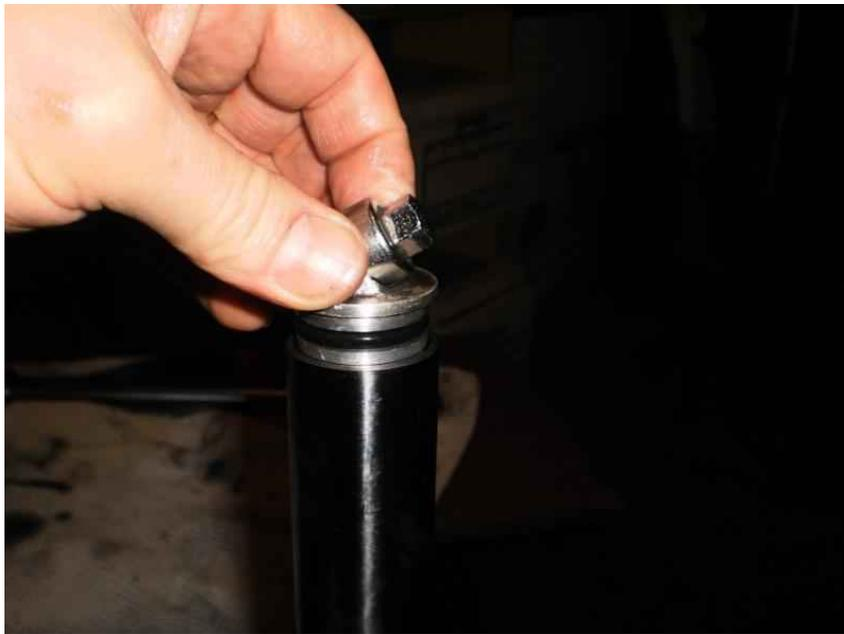
Remove the fork caps, spacers, washers, springs, and pour out the old fork oil. If you can hang the forks upside down for a while it will allow most of the oil to drain. Here you see the fork cap O-ring that can be replaced at this time.
