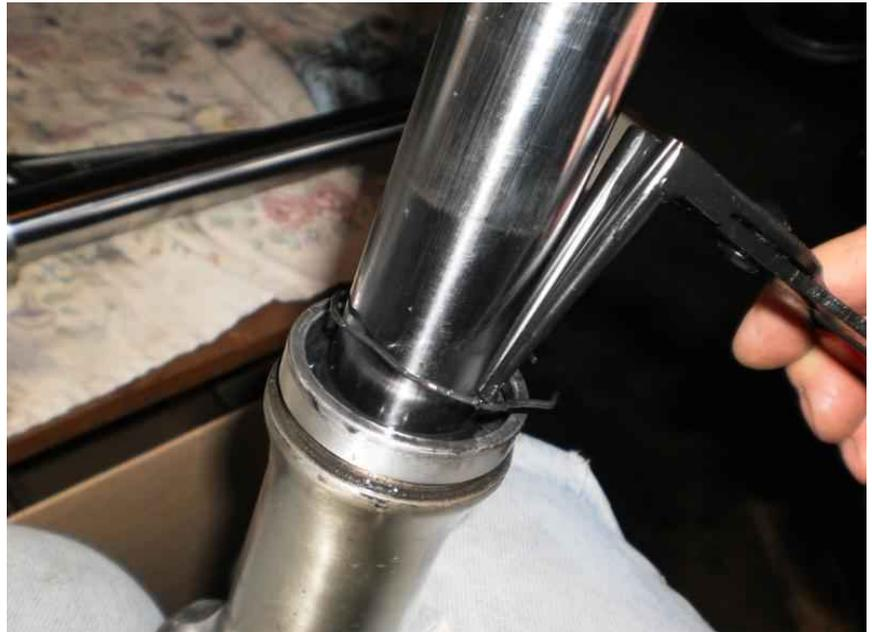
At this point I put the fork cap back on and hooked up my bicycle pump. The gauge on the pump maxed out at 174 psi. I pressurized the forks past that mark until the seal popped. It must've taken 180-200 psi to pop out the seal. A high-volume, high-pressure air compressor would come in handy here. But my bicycle pump worked. Sometimes it can take a few minutes, or hours, for the seals to pop. Be patient.
