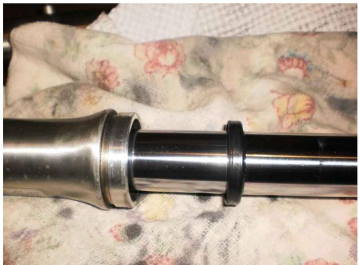
Next I used a 2 foot length of thick PVC pipe, I think it was  $1\frac{3}{4}$  inch in diameter, to push the new fork seal in place.
