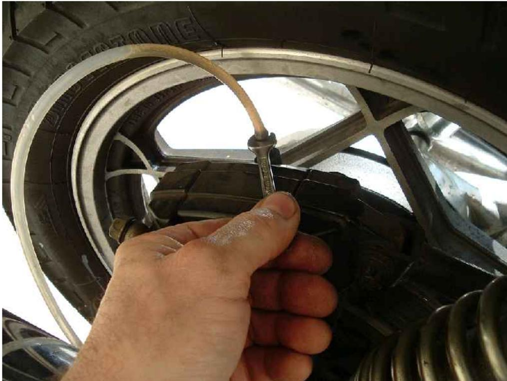
I remove the hose with a shop rag so as to catch any drips before they fall on the rotor. A well-lubricated rotor does not stop as well as a dry one.
