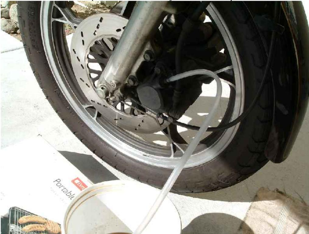
Then do the "pump/hold/loosen/squeeze/tighten" dance until all of the bubbles are gone or the fluid is replaced. This is what I started with:
