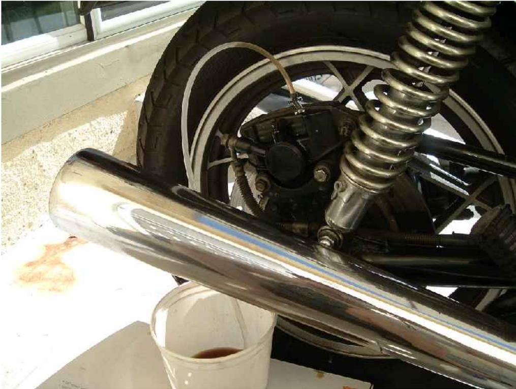
I pump the rear brake pedal to build up pressure and then hold it while I loosen the screw. The pedal goes down, the old fluid and bubbles come out, I hold the pedal down until I tighten the screw so as not to suck any air back into the system.
