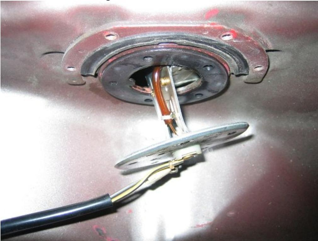
Here is the tricky part. You need to remove the sending unit from the tank without damaging the gasket. The float arm is about 10" long, and the electrics are in a housing that barely fits through. Try not to force it much, and fiddle it around until you can pull it through.
