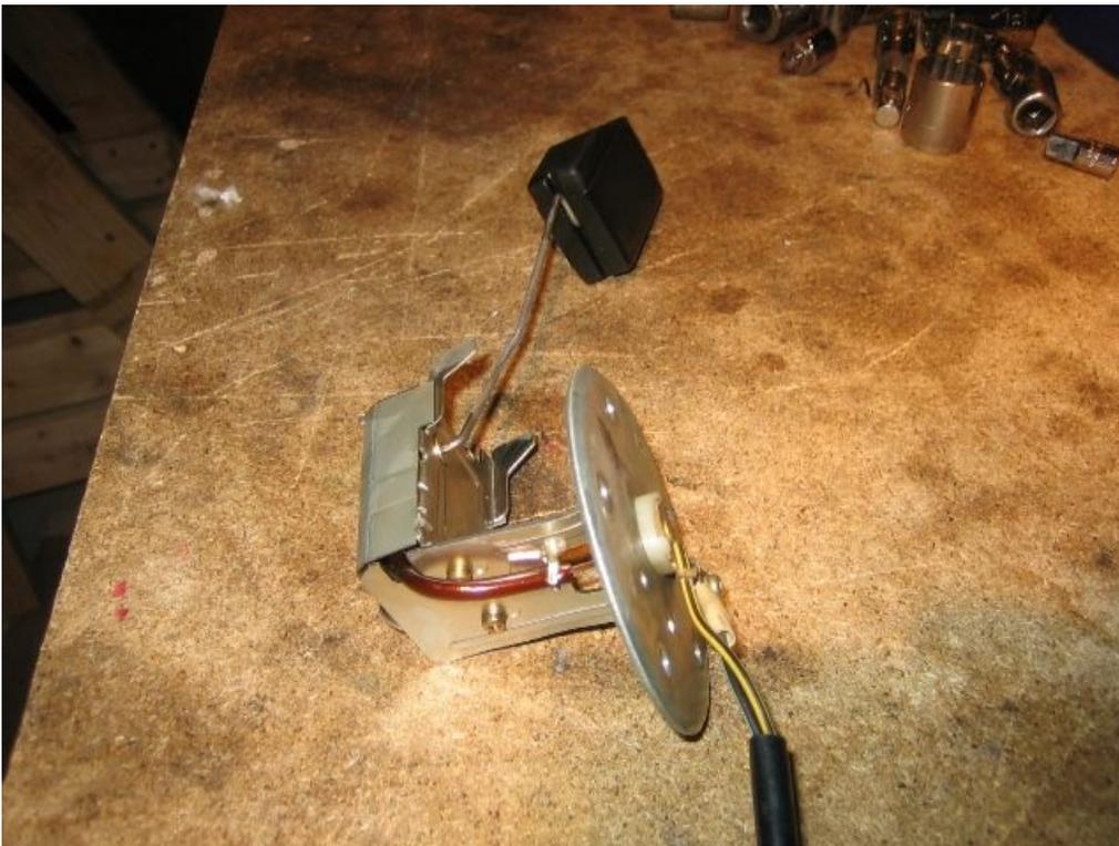
Next, you need to remove the cover to the guts of the sending unit. This picture shows the small tabs you need to bend up with a small screwdriver to take the cover off:
