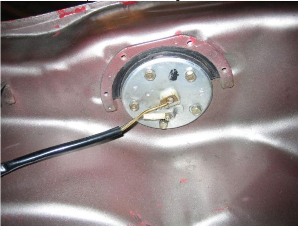
Make note of the position of the backer plate in relation to the tank. It needs to go back in exactly this position. If there is no alignment mark, use a Sharpie to make a line on the sending unit and the tank so that it can be realigned. Remove the 5 8mm bolts to free the sending unit.
