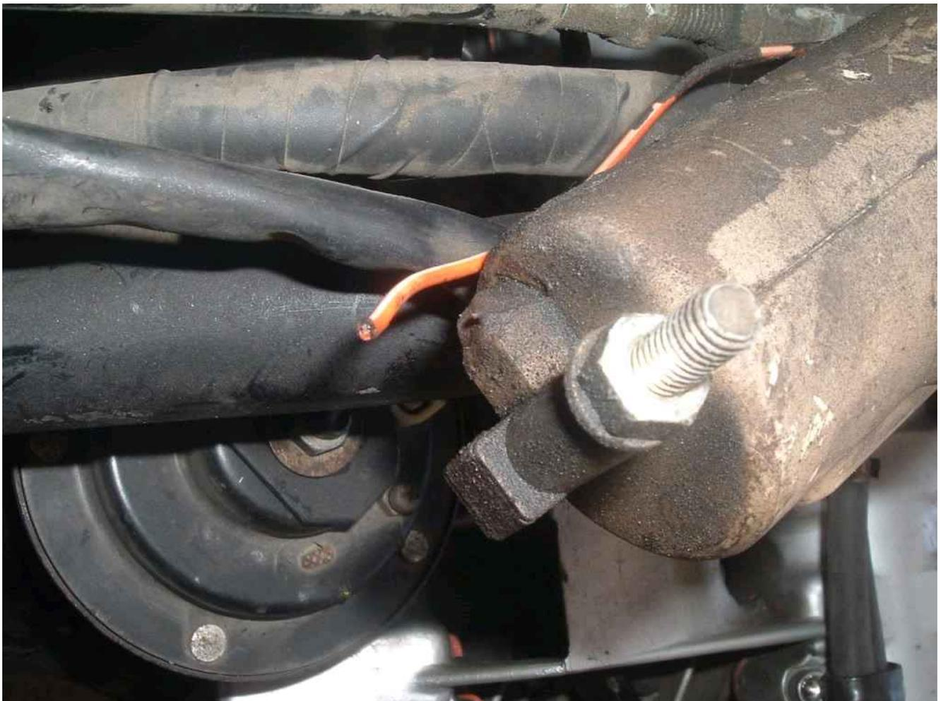
The 12v supply wire to the coil had broken loose. I wasn't sure if I could re-attach it or if I had to buy new coils. I decided to clean it up and find out. After I cleaned the area I found there was some epoxy over the connection. I carefully chipped it away with an exacto knife and discovered the solder terminal underneath.
