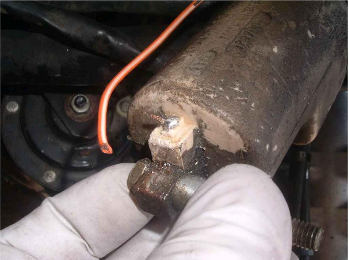
It seems that some Suzuki coils are different than others. Some coils have spade connectors, some have solder terminals. I got out my trusty soldering iron to clean up the terminal.
