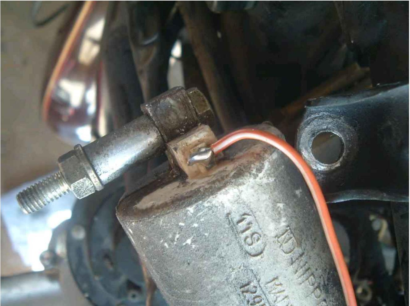
OK, the connection is good. Now I need to support it somehow, some kind of strain relief so that it is less susceptible to vibration or pulling.
