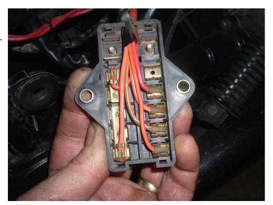
From here you can start disassembly. Remove the fuses and the contacts just snap out.
