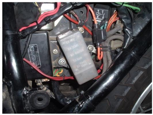
Remove the two screws to either side, disconnect the fusebox from the battery box, pop off the top cover and this is what you see.
