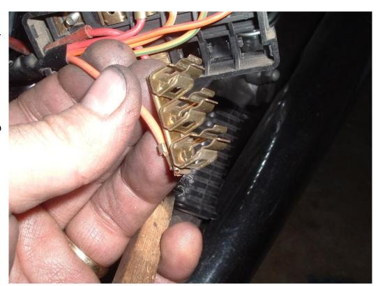
The main positive and negative inputs have a little different contact arrangement. Take out the screws and the contacts pop out for cleaning.
