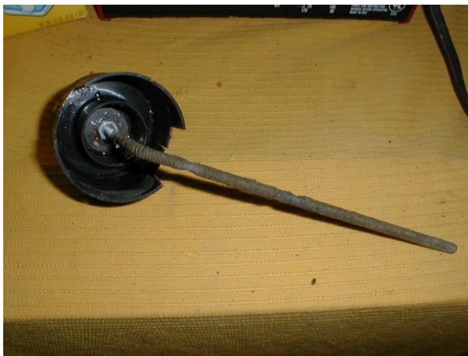
The positive clamp from the charger goes to the anode, the negative to the item to be cleaned, in this case, the tank itself. To connect to the tank, I first measure the inside diameter of the petcock opening – about .600 if memory serves. I picked up a rubber “cork” at Lowes that was about this .600 size in the middle of the cork taper. I pushed the rubber cork/plug into the petcock opening, good and tight. Of course the tank has to be sealed before the electrolyte is added.
