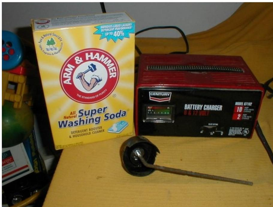
The anode is simply a piece of ¼ inch threaded rod (zinc plated) that I bent into shape to fit into the tank WITHOUT touching the sides (most important!). Note that the anode doesn't have to be plated, any cheap steel – or even stainless, will do. I simply had this rod around so I used it. Note the threading was an advantage as I could use nuts to mount the rod to the plastic cap.
