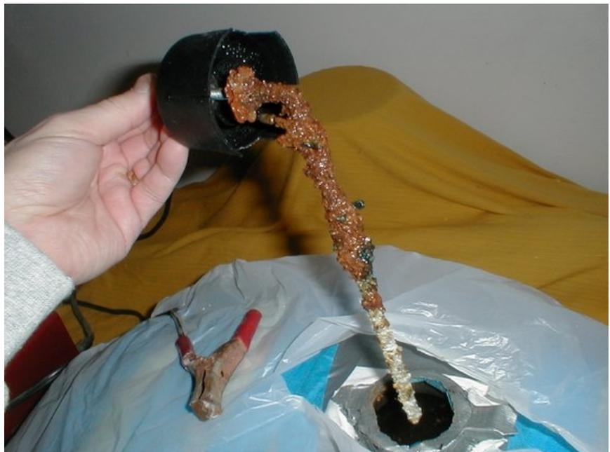
The second photo shows the basic equipment; a battery charger, the (freshly cleaned) anode and the mix for the electrolyte. The Arm & Hammer product wasn't particularly easy to find, but I eventually tracked it down at a very large mega-superstore (Meijers). It's cheap so I bought two boxes – just to be sure I have a future supply.
