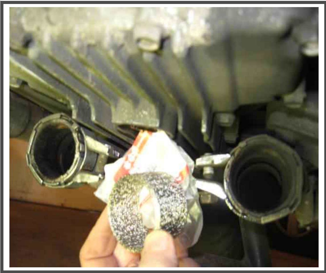
This picture shows the exhasut pipes off, with original connectors in place. I am holding one of the new connectors. New connector seems to be all metal braid.
