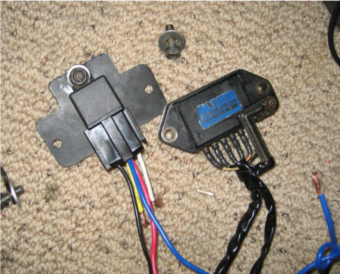
Final mount location at the battery box replaced the OEM ignitor. The green connector is 4 pin goes to the Dyna-S. The relay shares a left hand mount with a blow by collection bottle.
