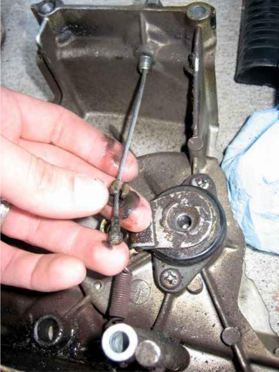
5. Unscrew and remove the cable from the cover. Now is a good time to clean the crud out of the cover!
