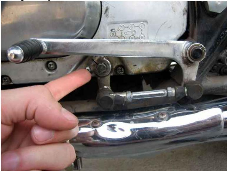
Remove the shifter cover. I had to use an impact driver to loosen a few of these.
