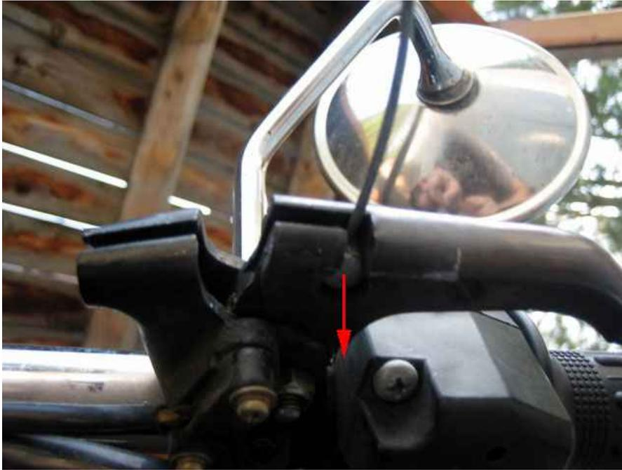
4. Detach cable from cover. Rotate as shown until there is enough room to slide the nut out.
