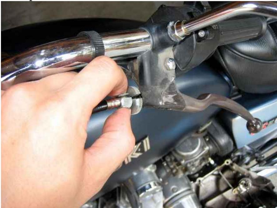
With the adjuster bolt out, rotate the cable out of the slot and slide it down to free it.
