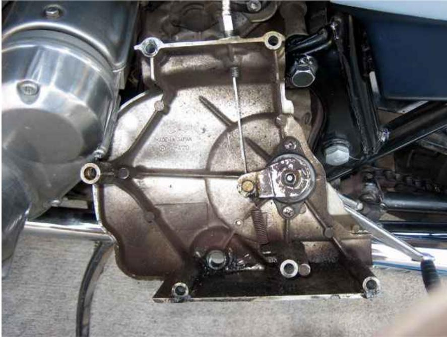
3. Detach cable from clutch lever. Unscrew and remove: the slots in the bolt and nut line up to free the cable.
