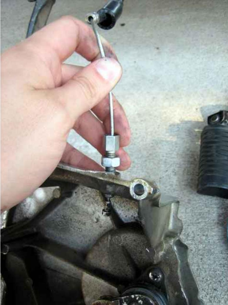
6. Note the routing of the old cable then remove it. Removing the gas tank is optional, but it does give you some extra room.
