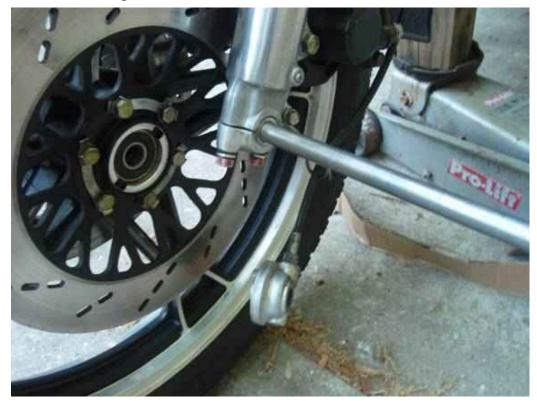
To get the wheel all of the way out, I had to remove one of the calipers. I removed the two "7" marked bolts from the fork.
