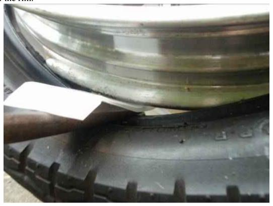
Insert your other tire iron 2 inches away and push down. Remember to use a rim protector. **Note:** Here I'm being paranoid and using 2 rim protectors. One is sufficient.
