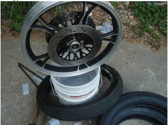
Take the time now to clean the area on the rim that holds the bead with a Scotch-Brite. This will get all of the old rubber off and ensure a good seal with the bead.
