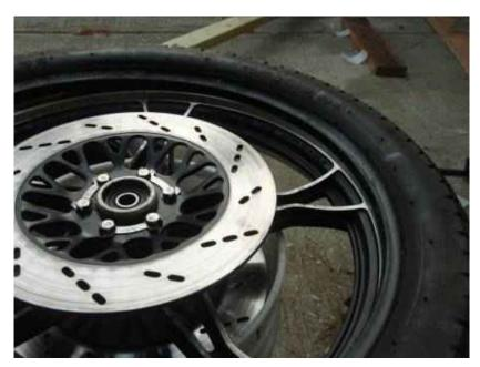
Go ahead and flip the tire over and put a rim protector between the rim and tire. This time, instead of pulling the tire OVER the rim, you're going to be pushing it BELOW the rim. Insert tire iron between the rim protector and push down. Make sure the rim protector is protecting the underside of the rim.
