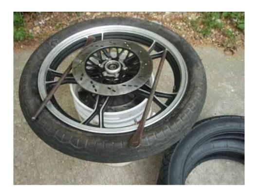
Place a rim protector in between the rim and tire. Stick your tire iron in between the protector and tire and wedge it against the rim.
