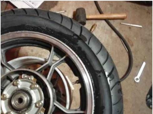
Now you need to inflate the tire, and quickly if you used soapy water. Set your compressor to about 60 psi even though you only go up to about 40. When I did my tires, I didn't have a good compressor tip that let a lot of air through. I should've used one that let more air through, like the one in the picture.
