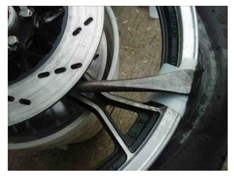
Insert your other tire iron with rim protector about 2 inches away from the first one and do the same motion. The other tire iron should feel a little loose now. Even if it doesn't, pull the first one out and put it in with a rim protector about 2 inches away from the other one. Again, with the same motion, pull the tire over the rim. As you get more tire off the rim, you can gradually move from 2 inches between irons to about 6 or 8 inches until one bead is off.
