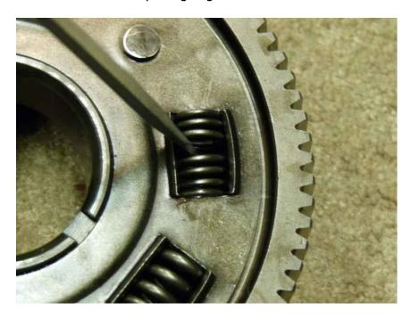
Rotate the spring in it's slot as you go, separate each coil a tiny bit.
