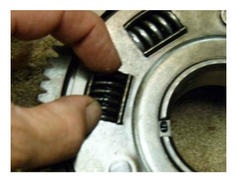
When the springs are getting tighter, they get harder to rotate. Put the screwdriver in between coils at one side of the opening, twist it and pull it across to rotate the spring. Keep going until all the springs are good and tight, try to get them all evenly tight, all the way around.
