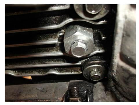
Future oil changes will involve using a large crescent wrench to hold the larger bolt stationary while using a small socket to remove the piggyback bolt and drain the oil.
