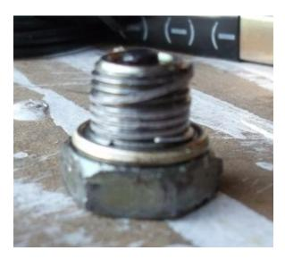
As you can see, the threads are now full of aluminum from the oil pan. The plug itself looks OK, the bolt is harder than the oil pan. But the oil pan threads have been stripped so that is where the repair must take place. There are several ways to repair stripped threads. One is to use something similar to a <a href="Fix-a-Thread Plug Saver kit">Fix-a-Thread Plug Saver kit</a>. This kit repairs the threads for a spark plug which is the same size (M14 x 1.25).
