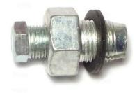
This is a "piggyback" drain bolt and can usually be found right alongside the single bolt (above) for about the same price. I chose this bolt so that I could leave the big plug in the pan and use the piggyback bolt to drain my oil. This would cause less wear and tear on the oil pan itself.
