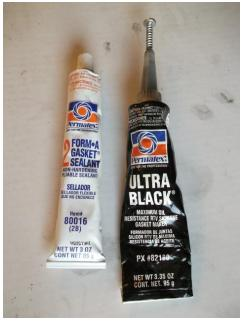
Instead of a liquid metal, like JB Weld, I used Permatex #2 on the threads of the big bolt. Since I eventually plan to use a TIME-SERT, this would allow extraction of the bolt without destroying the pan but provide a good seal. I also used the Ultra Black permatex on the smaller piggyback bolt since there is no washer or gasket.
