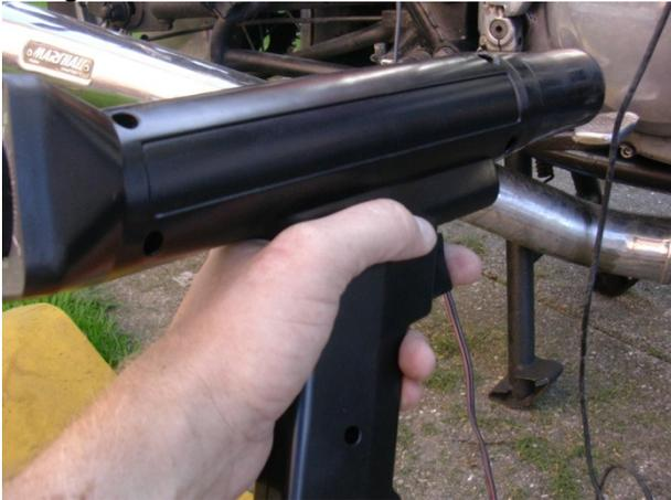
And it must be attached to one of the four ignition cables.
