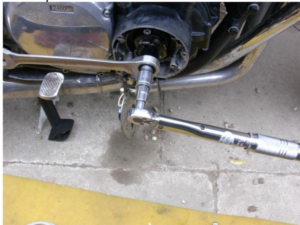
Fix the new base plate with the 3 screws you removed earlier. Remember to fix the old marker plate behind the new plate, and remember to place the hole in the base plate facing upwards, enabling you to see the top-mark.
