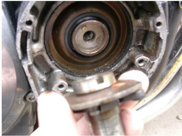
The advancer moves the point of ignition, when speed arises – by spreading two weights (hold by springs) due to centrifugal force. Spread the weights by hand, and pull out the advancer unit.
