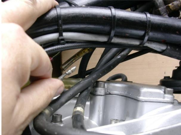
Connect the white and black wires in the same way the old wires were connected, and connect the red wire to a 12V switched with the ignition key. The orange wire to one of the ignition coils could be used.
