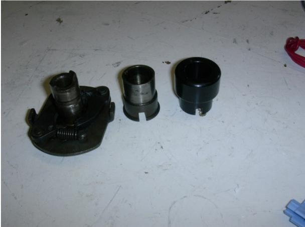
The new rotor is shown to the right, and the old eccentric guide in the middle. Oil the axel of the advancer, pull out the weights, and mount the new rotor. With the advancer placed with 1-4 marks facing upwards, the little magnet in the rotor should face left
