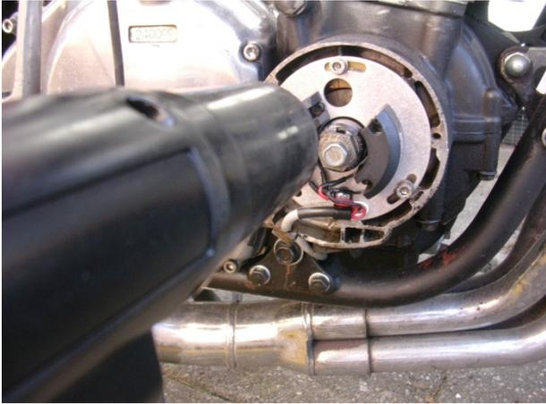
The mark should match the first 2-3 mark. If not, move the base plate. Raise the engine speed slowly. The mark should move smoothly, and by 2500 RPM, the mark should match the other 2-3 mark. Redo for 1-4, if necessary move the black pick-up. If the second mark is not met, at 2500RPM, check the advancer unit for correct function.
