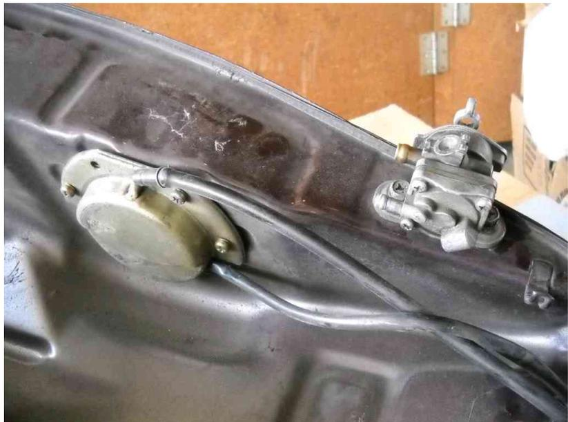
Once you remove the fuel gauge send unit overflow plate you will see the the send unit connectors.
