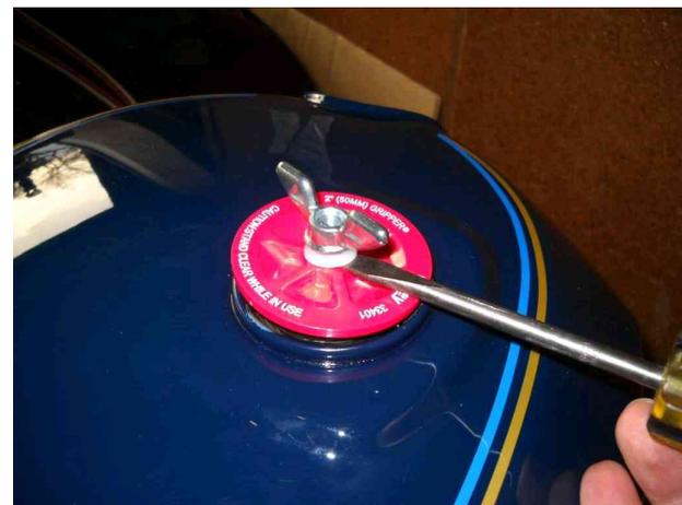
Here we are, with our Evapo-Rust and nails inside the sealed tank.
