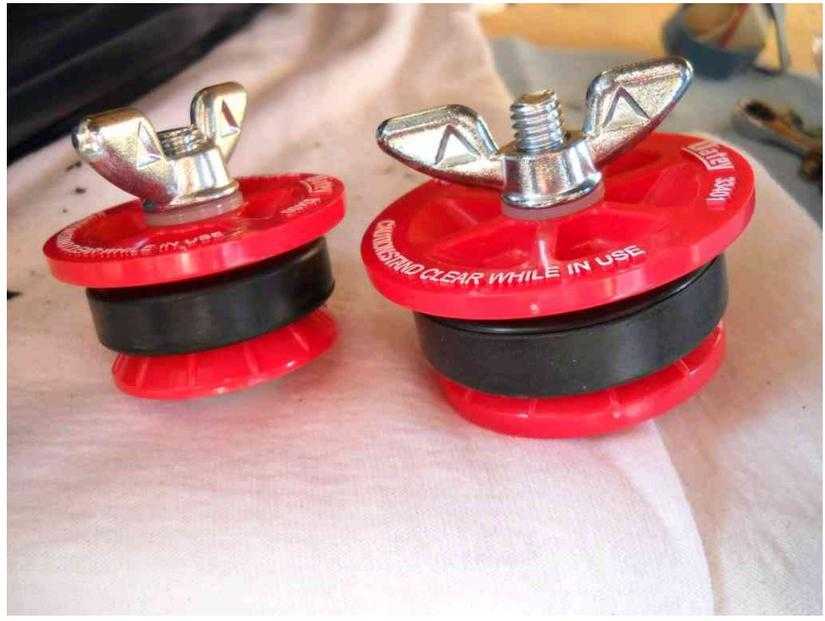
The plug for the send unit hole went right in and fit nicely. Tightening the wing nut squeezed the rubber ring and made a good seal around the hole.
