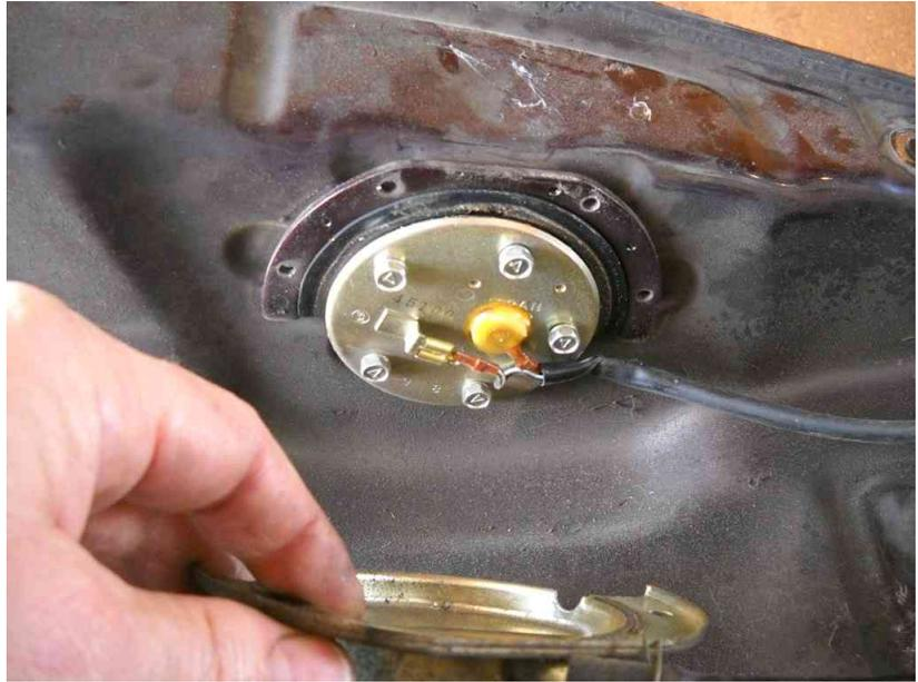
Remove the five bolts holding the send unit. I reused my gaskets and petcock O-ring but next time I am definitely getting new ones.
