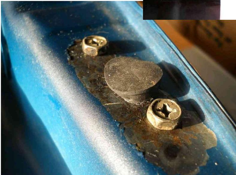
I used a regular rubber stopper for the petcock hole and put the bolts back in the bolt holes. I couldn't find rubber stoppers big enough for the other holes. But here's what I did find...
