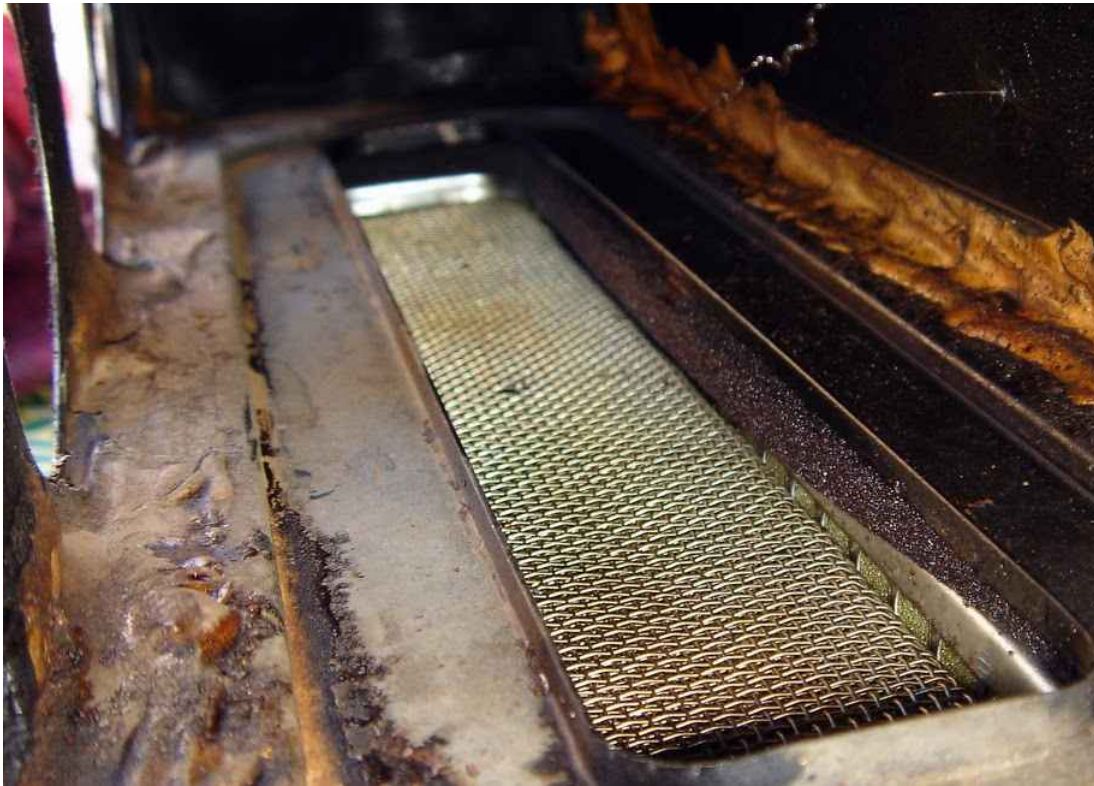
3) The air filter gasket seems to be trying to escape on the right side of this picture.
