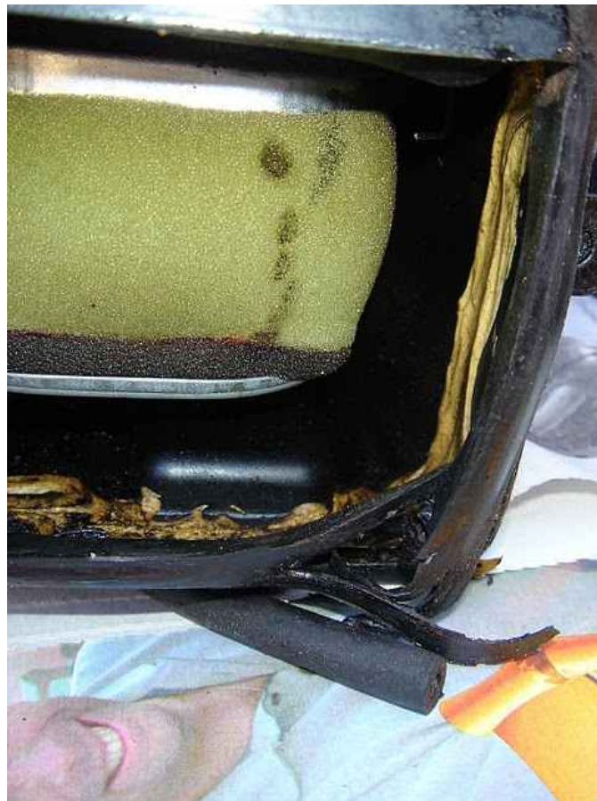
4) The corner of the rubber seal is just shredded on this side.
