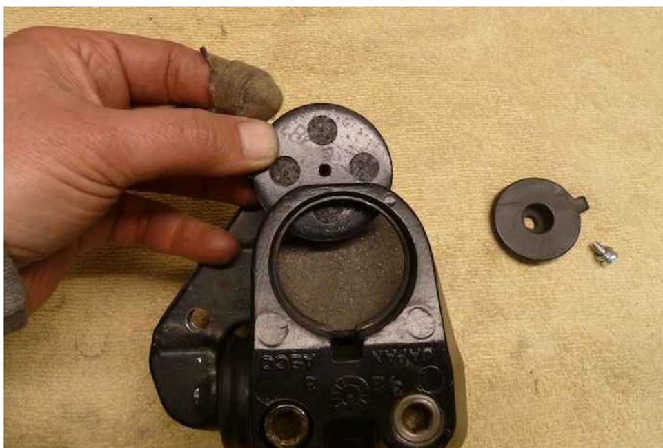
Once the inside pad is properly seated in its place in the caliper, secure it with a 5mm bolt through the back of the plastic hatch. Voila, your calipers are done and ready to be remounted to the forks!
