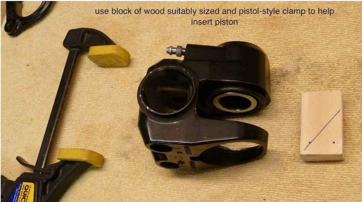
A suitably sized block of wood (approx  $\frac{3}{4}$ " x 3" x  $1\frac{1}{4}$ ") gives the clamp the needed reach through the caliper body. Using the pistol-style clamp push the piston all the way into the cylinder. The inner ridge of the piston boot normally pops into the groove at the top of the piston once the piston is all the way in. (make sure this happens).
