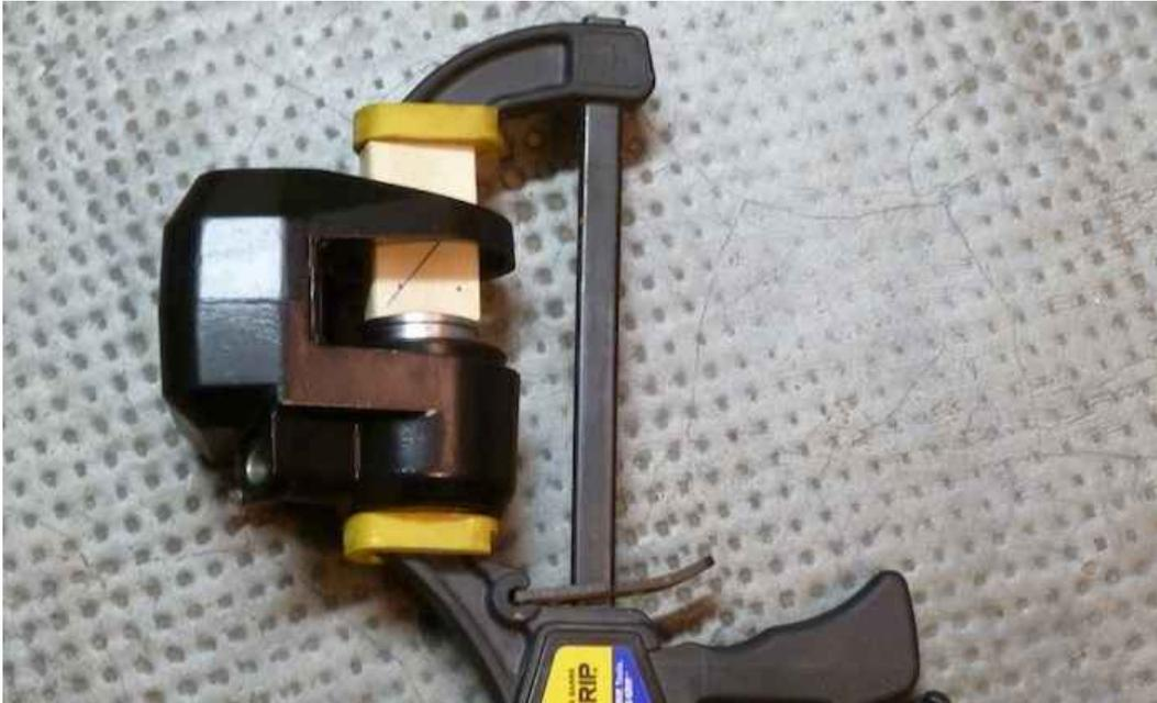
The next step is to pre-install a new dust boot on the mounting bracket. I found a little petroleum jelly helped get the boot sliding along the bracket body.
