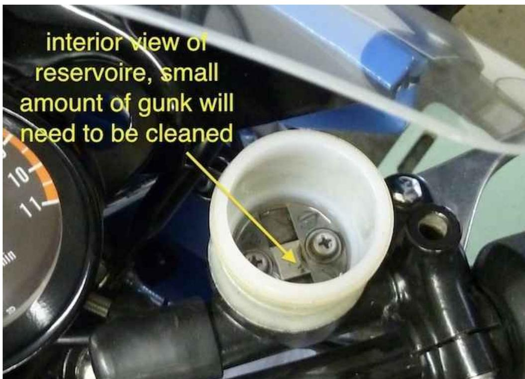
To remove the remaining fluid in the brake lines, place the cap temporarily back on the reservoir (don't bother with the diaphragm for now) and get a hold of your pickle jar and lines. Connect the lines to the nipples atop the breather screws.
