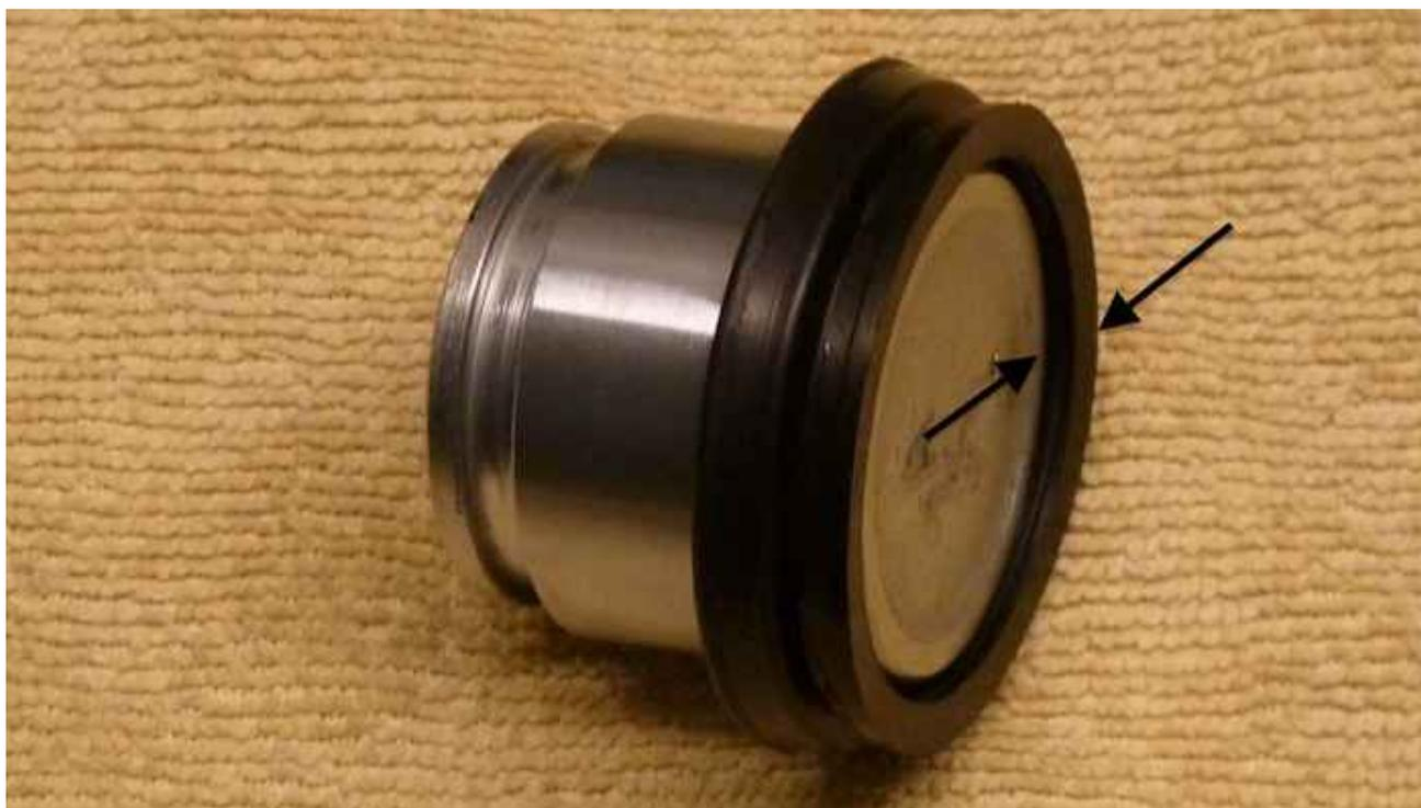
Once your piston & boot assembly is properly fitted into the cylinder it should look like the picture below. Double check that the piston boot is properly fitted and give the sides of the piston a *thin* coat of clean brake fluid to facilitate the next step.
