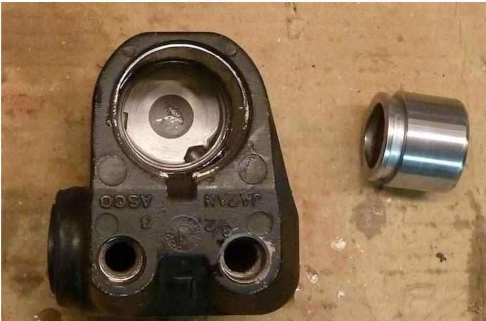
Next remove the piston seal from inside the cylinder. A dentist's pick works great for this, but the tip of an Exacto knife will work too. Whatever method you use, be careful not to score the cylinder walls.
