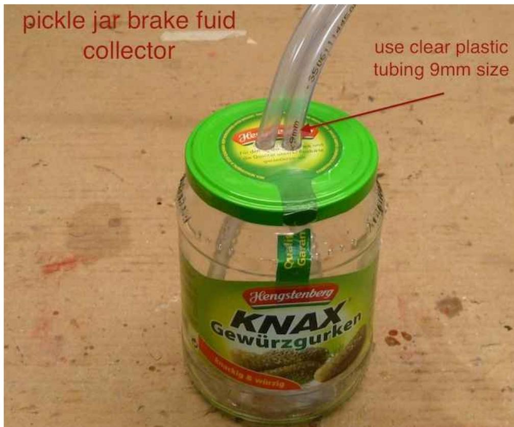
Before the calipers can be removed from the bike, all the brake fluid must be drained from the system. I found it practical to start by opening the reservoir on the front master cylinder and draining its contents with a syringe.
