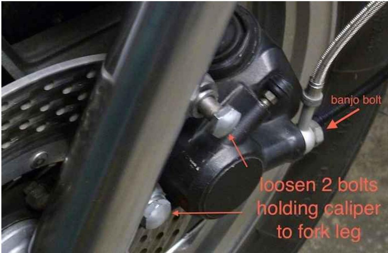
Once the banjo bolt has been removed check it for any gunk clogging up its passages.
