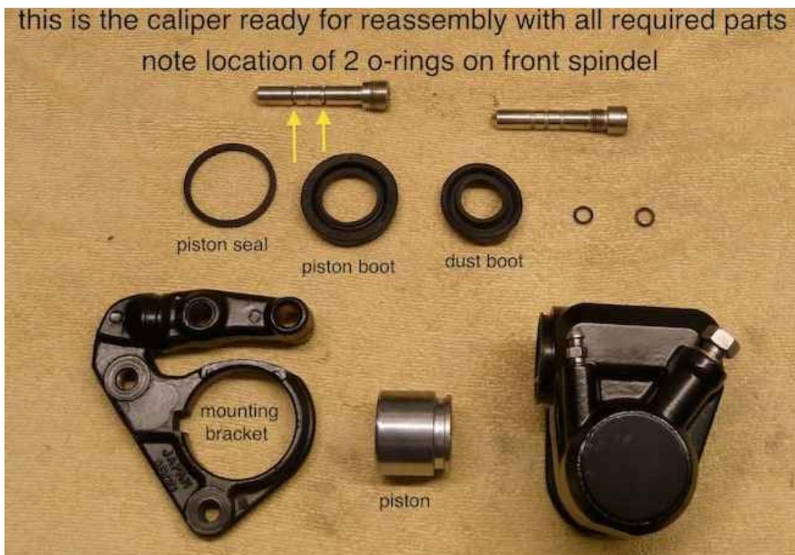
First, take a new piston seal and give it a thin coat of clean brake fluid. Now place the piston seal inside the groove for it in the cylinder wall. Start at any one point in the cylinder wall groove and work your way around with your fingers until it's all in. Next, use an old ¼" paint brush and give the whole cylinder a light coat of clean brake fluid.
