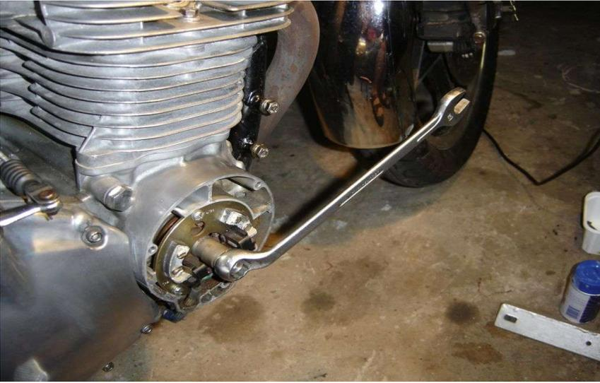
Use a 19mm spanner and turn the engine clockwise until the the highest part of the cam lobe on inlet #4 is perpendicular to the valve and it is thus fully opened.
