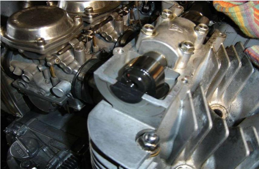
Now insert the “valve tool” at about 10 o'clock in the spark plug hole and push the folded part of the cable tie between the open valve and the head. You should be able to see the edge of the valve once it is open, if you shine a light into the spark plug hole.
