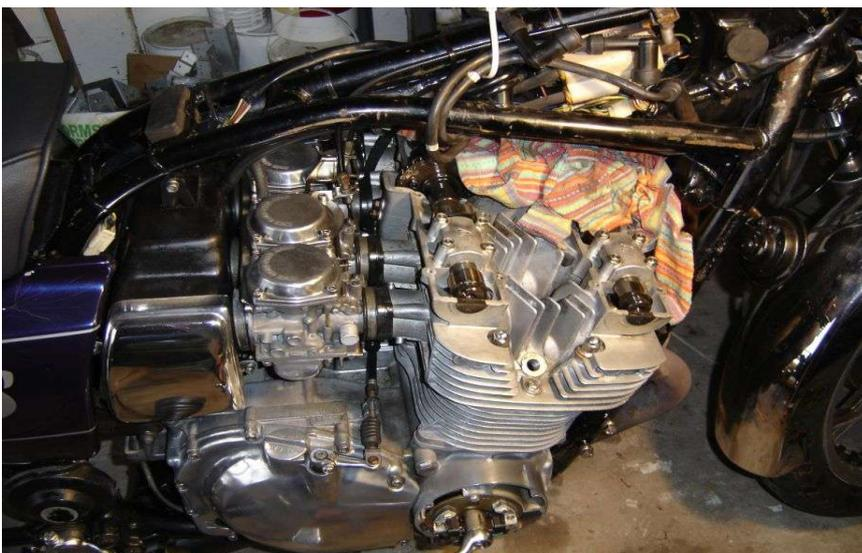
Remove tank, plugs, tie back plug leads, remove valve cover and timing cover.
