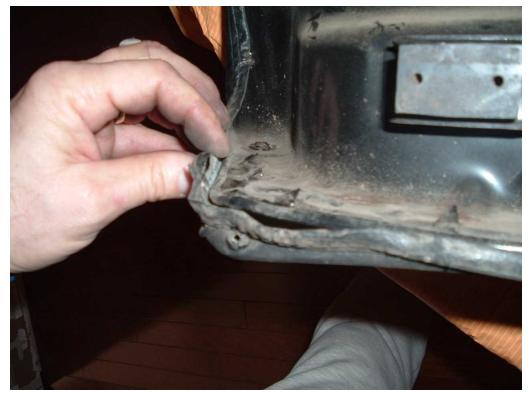
Here's a view along one side showing the hooks and clips after the cover is loose.
