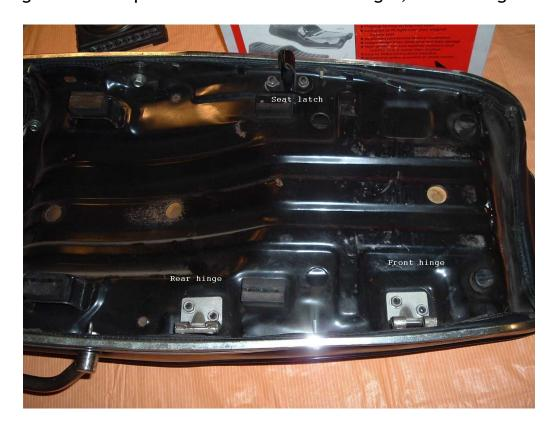
Here's some of what you'll see under the seat; hooks and clips to hold the edge of the seat cover and the grab rail bolts.
