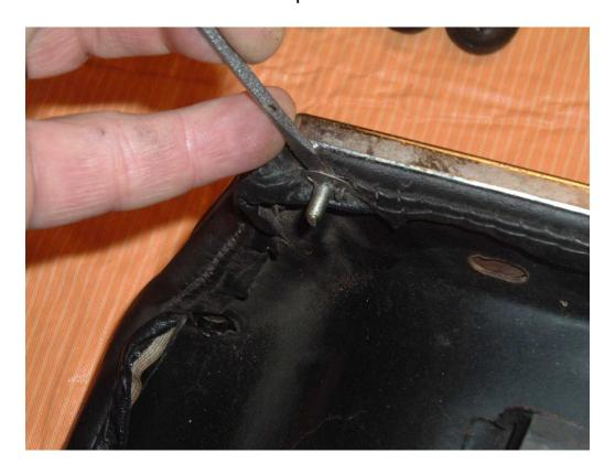
I broke two before I realized that I must pry a couple of the tabs up before they come off. Doh! I used a pair of wire cutters to pry up a couple of tabs, then the nuts
