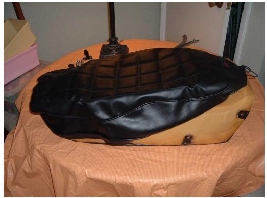
Start at one end and work your way toward the other going back and forth from side to side, pulling and tucking. I found it easier to put the seat upside down in my lap while fitting the cover.
