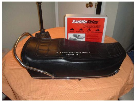
The fist thing I did was flip it over and remove the hinges, latch and grab rail.
