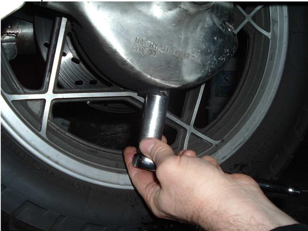
Here's a shot of my small container catching the old gear oil. I poured this into my regular oil change receptacle so that I could recycle it along with my engine oil.
