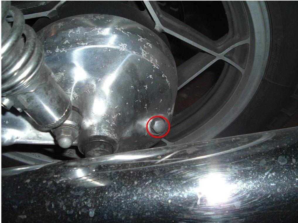
Here is a picture of the final drive drain plug.
