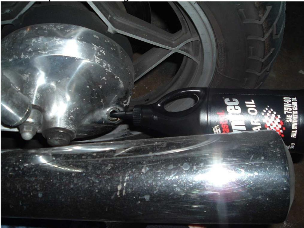
Just fill it up to the bottom of the fill hole threads. If it starts leaking out, that means it's over full.
