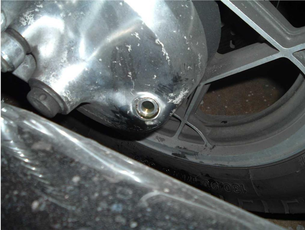
Next I take off the drain plug (same size as spark plug). Have a container handy to catch the oil.
