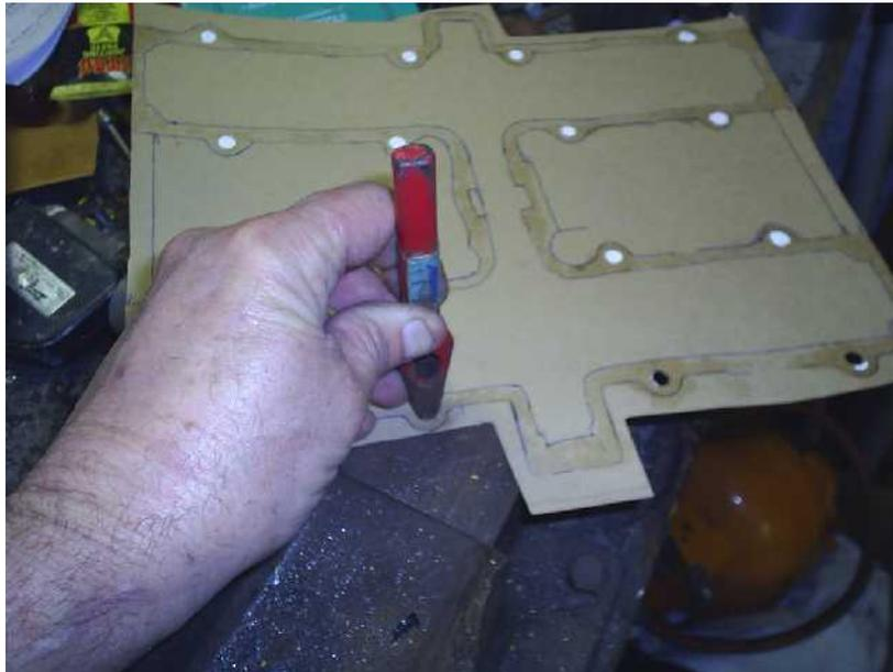
10. The 2 holes diagonally opposite each other which had dowels in them to locate the cover on the cylinder head had to be made a bit larger (next size up hole punch).
